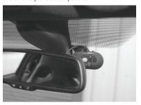
The adhesive mount supplied with the camera uses a VHB 3M adhesive pad. Remove the red sticker from this mount
