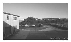
The RoadHawk Ride camera embeds the time and date on to any video being recorded. In order to set the time and date you need to put a file on to the SD card so the camera can be set accordingly.
